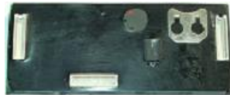
Figure 4. SecureD FPGA Sample (back) – Epoxy Coated
