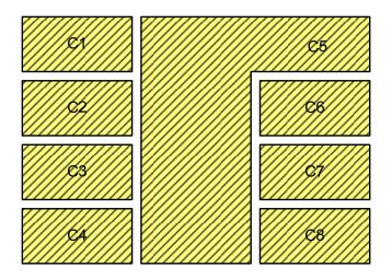
Figure 2 – Contact Plate Example – Contact Physical Interface
