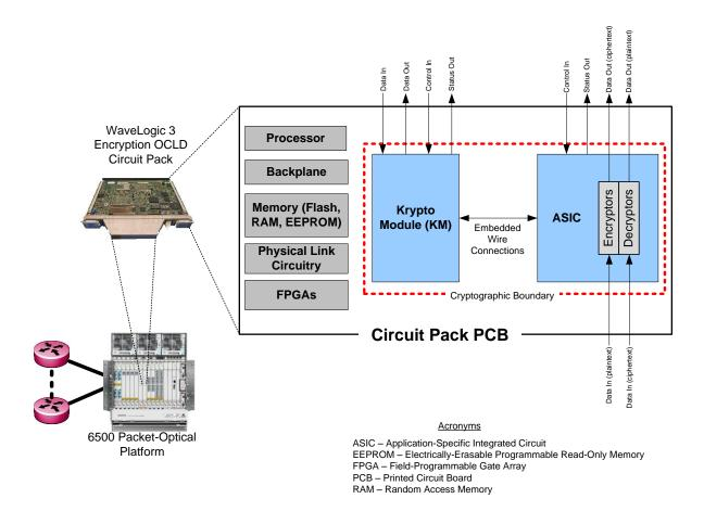
Figure 3 – Module Block Diagram
