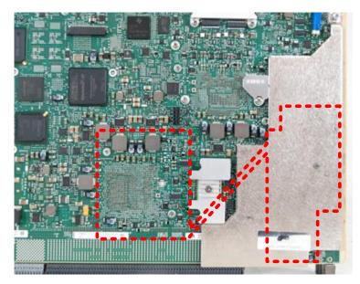
Figure 2 – Module on Circuit Pack (Bottom View)
