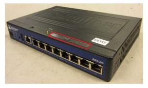
Figure 15: SRX100 Tamper-Evident Seal Placement- One Seal
