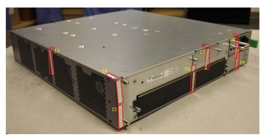
Figure 21: SRX550 Tamper-Evident Seal Placement on Rear and Left Side- Seven Seals
