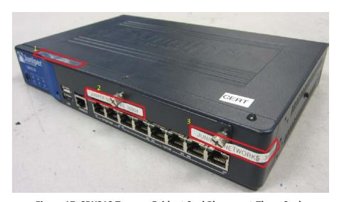
Figure 17: SRX210 Tamper-Evident Seal Placement-Three Seals
