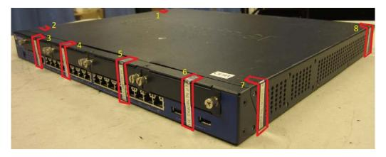
Figure 19: SRX240 Tamper-Evident Seal Placement-Eight Seals
