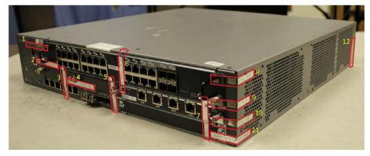
Figure 20: SRX550 Tamper-Evident Seal Placement on Front and Right Side-Twelve Seals
