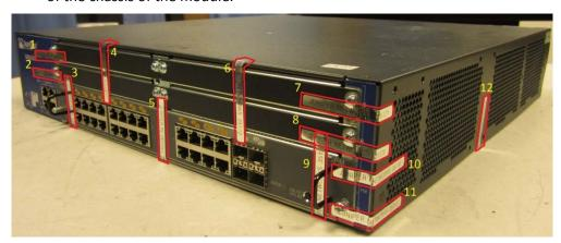
Figure 22: SRX650 Tamper-Evident Seal Placement on Front and Right Side- Twelve Seals
