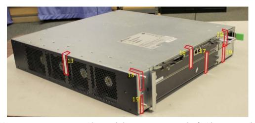
Figure 23: SRX650 Tamper-Evident Seal Placement on Rear and Left Side- Seven Seals
