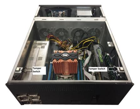
Figure 10: tamper switch
