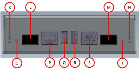
Figure 4: IAS KG-RU Front Panel Ports and Interfaces
