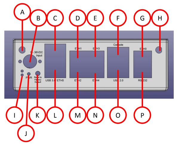
Figure 1: IAS Router Micro Port and Interface Identification
