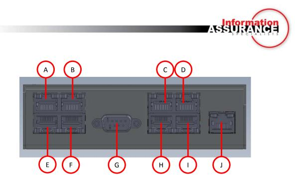
Figure 3: IAS KG-RU Rear Panel Ports and Interfaces
