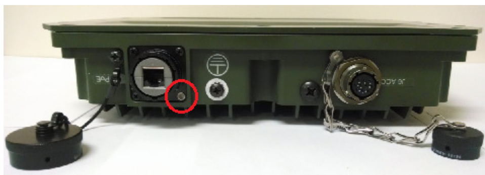
Figure 4 – Tamper-Evident Pin Location for RF-7800W
