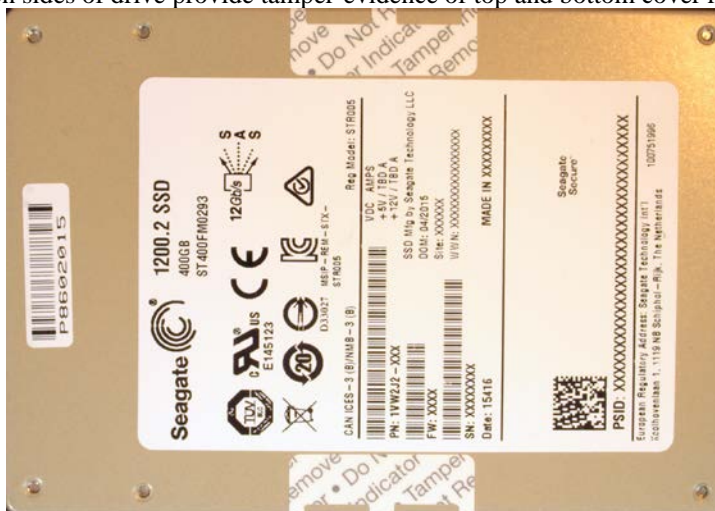
Figure 1: Top view of tamper-evidence label on sides of drive
