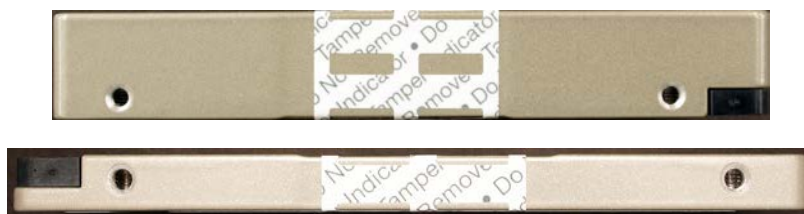
Figure 3: Right-side view of tamper-evidence label on right side of drive
