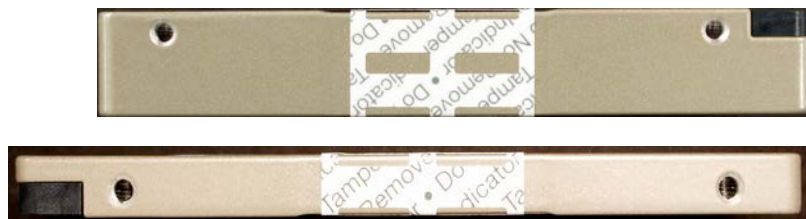
Figure 2: Left-side view of tamper-evidence label on left side of drive
