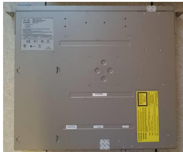
Figure 48 ASA 5515-X Bottom TEL Placement
