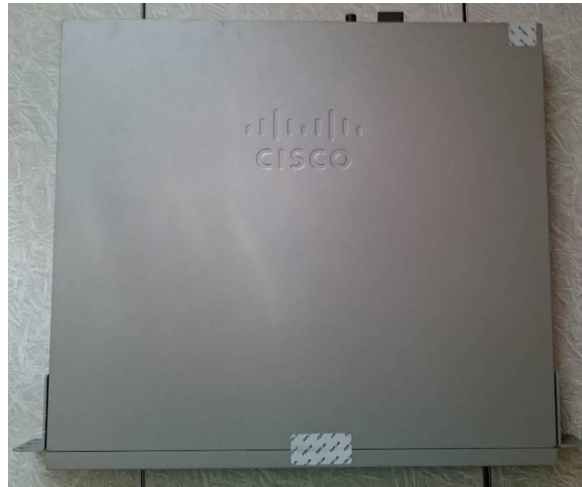
Figure 47 ASA 5515-X Top TEL Placement
