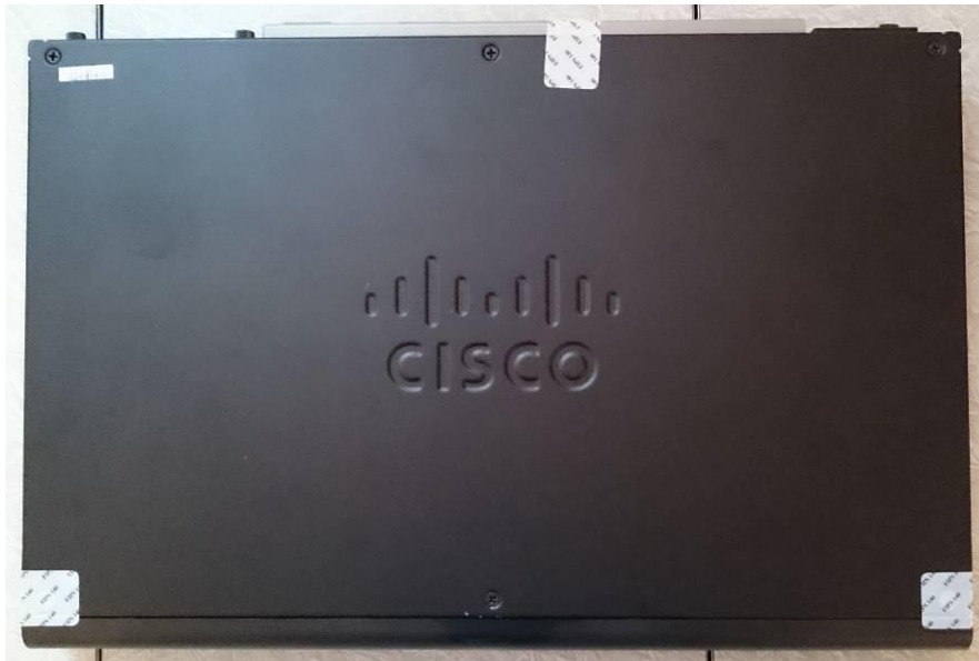
Figure 53 ASA 5516-X Top TEL Placement
