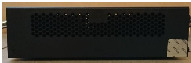
Figure 28 ASA 5506H-X Left Side TEL Placement
