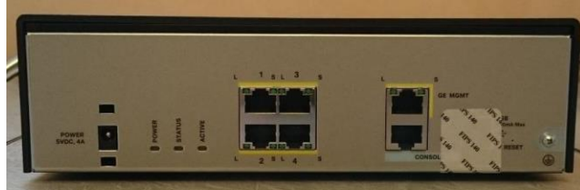
Figure 27 ASA 5506H-X Rear TEL Placement
