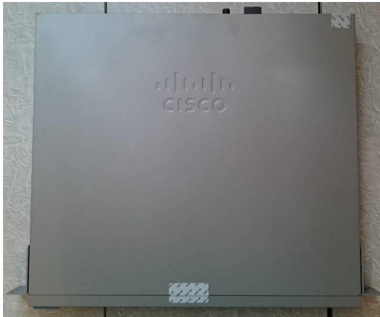
Figure 59 ASA 5525-X Top TEL Placement
