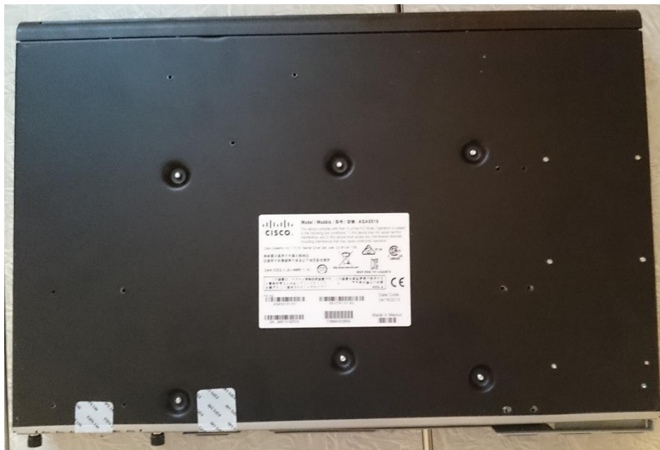
Figure 54 ASA 5516-X Bottom TEL Placement
