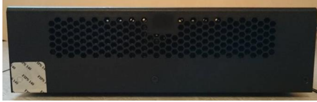
Figure 26 ASA 5506H-X Right Side TEL Placement
