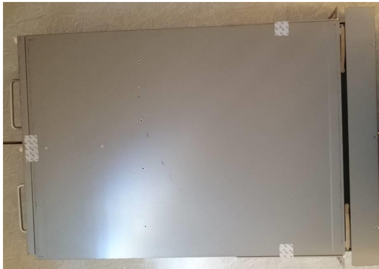
Figure 75 ASA 5585-X Bottom TEL Placement
