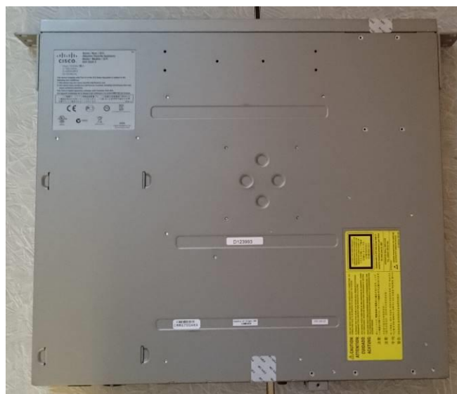
Figure 60 ASA 5525-X Bottom TEL Placement
