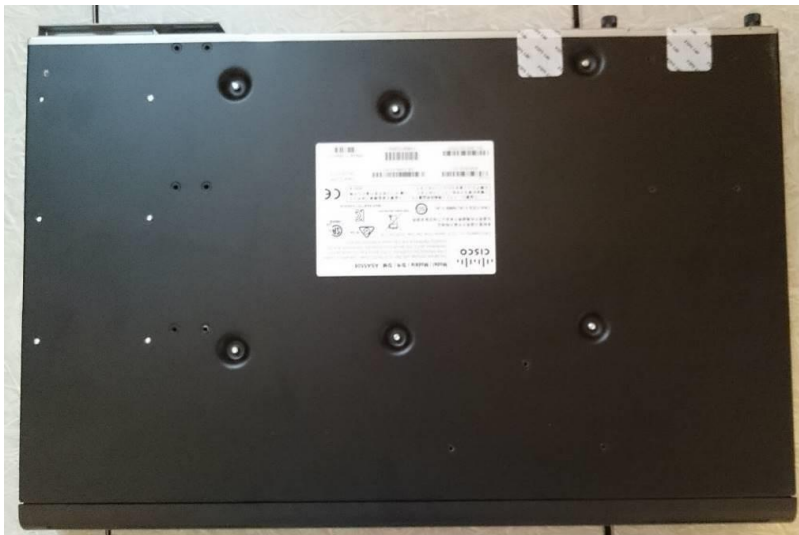
Figure 36 ASA 5508-X Bottom TEL Placement
