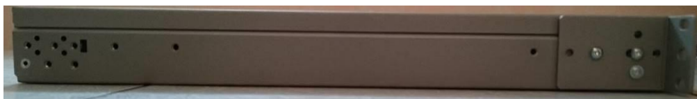
Figure 58 ASA 5525-X Left Side TEL Placement
