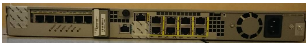
Figure 57 ASA 5525-X Rear TEL Placement
