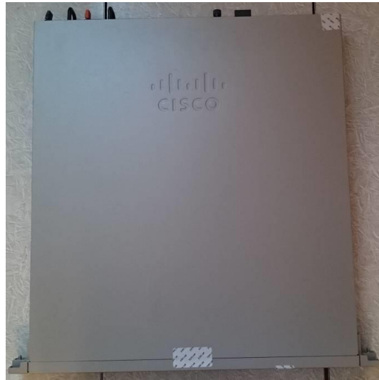
Figure 71 ASA 5555-X Top TEL Placement
