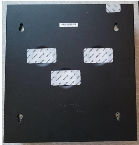
Figure 24 ASA 5506-X and ASA 5506W-X Bottom TEL Placement
