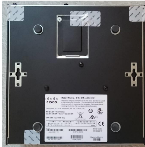
Figure 30 ASA 5506H-X Bottom TEL Placement
