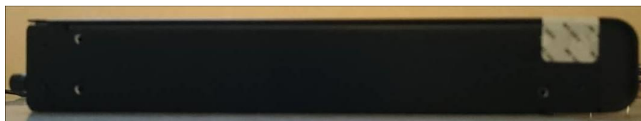
Figure 34 ASA 5508-X Right Side TEL Placement
