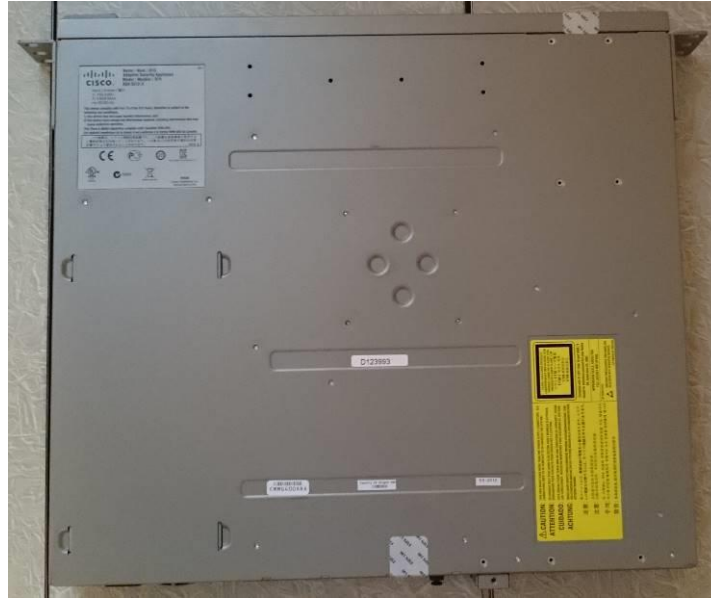
Figure 42 ASA 5512-X Bottom TEL Placement
