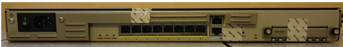
Figure 50 ASA 5516-X Rear TEL Placement
