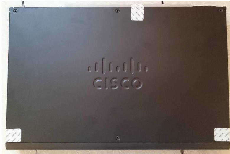
Figure 35 ASA 5508-X Top TEL Placement
