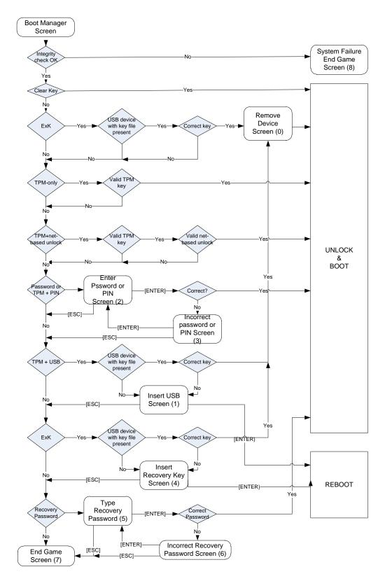
Figure 3 Flow Logic
