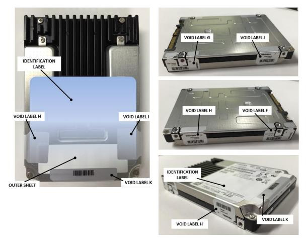
$<sup>^3\,</sup>$  OUTER SHEET is an opaque seal covering some holes of the top cover. It cannot leave "VOID" message, but leaves the evidence of the cut.
