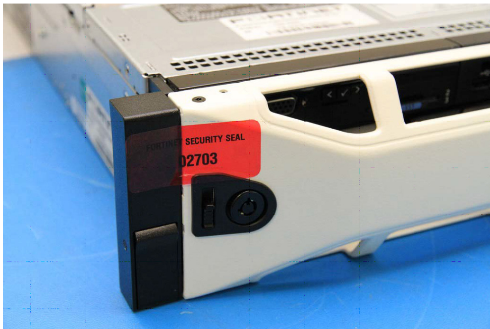
Figure 7: FortiManager-4000D Front Faceplate seal
