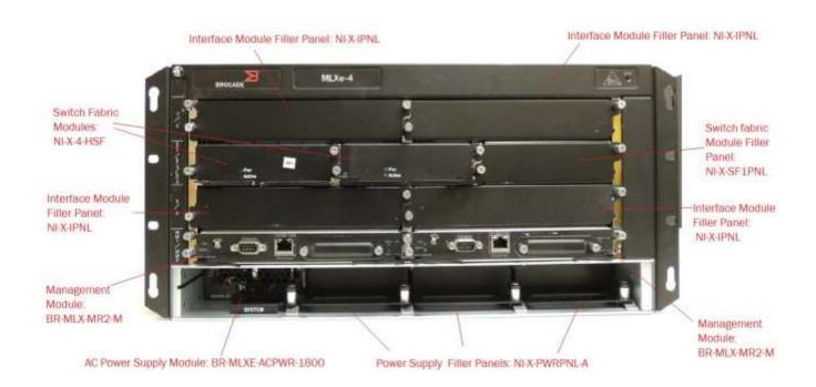
Figure 6 MLXe-4 Cryptographic Module with Chassis: BR-MLXE-4-MR2-M-AC backside
