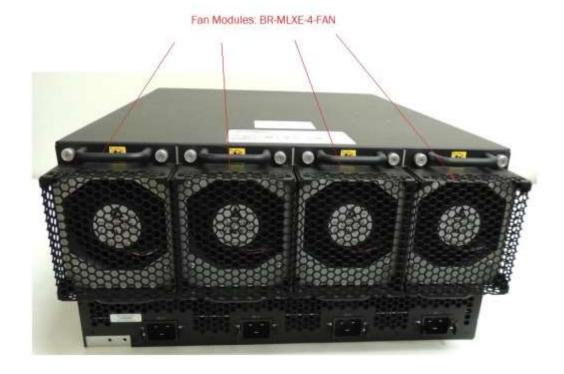
Figure 3 MLXe-4 Cryptographic Module with Chassis: BR-MLXE-4-MR-M-DC (DC Power Supply)
