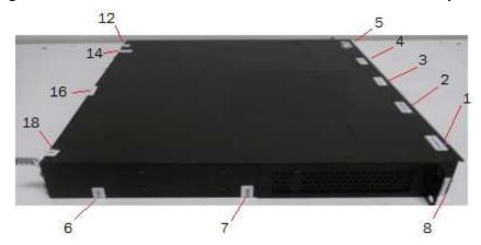
Figure 105 Rear view of a Brocade CES 2024C-4X device with security seals
