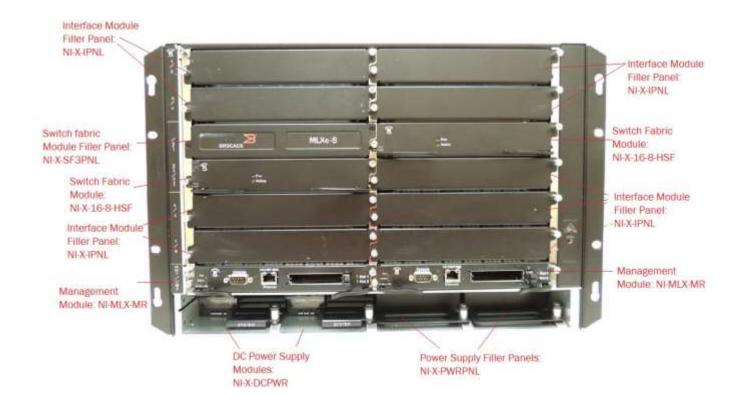
Figure 12 MLXe-8 Cryptographic Module with Chassis: BR-MLXE-8-MR-M-DC backside
