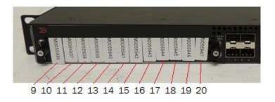
Figure 86 Rear, top and left side view of a Brocade NetIron CER 2024F device with security seals
