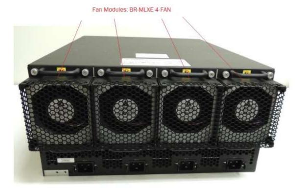
Figure 9 MLXe-8 cryptographic module with Chassis: BR-MLXE-8-MR-M-AC (AC power supply)
