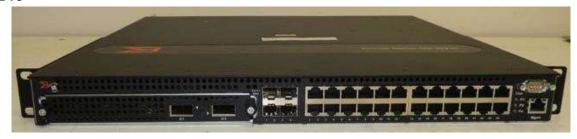
Figure 48 NI-CER-2024C-ADVPREM-DC backside with Interface module: NI-CER-2024-2X10G with Power supply RPS9DC (DC Power Supply)
