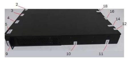
Figure 104 Left side view of a Brocade CES 2024C-4X device with security seals
