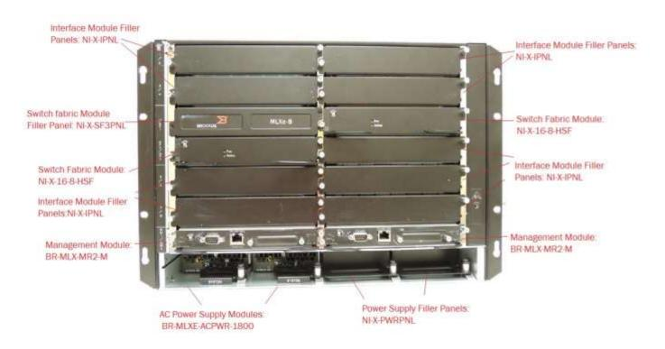
Figure 14 MLXe-8 Cryptographic Module with Chassis: BR-MLXE-8-MR2-M-AC backside
