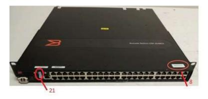
Figure 90 Right view of a Brocade NetIron CER 2048 device with security seals
