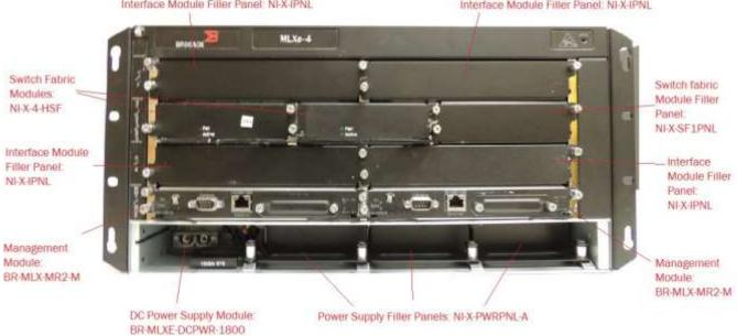
Figure 8 MLXe-4 Cryptographic Module with Chassis: BR-MLXE-4-MR2-M-DC backside
