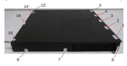
Figure 110 Rear view of a Brocade CES 2024F-4X device with security seals
