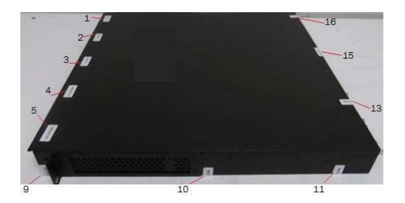
Figure 94 Left side view of a Brocade CER 2024C-4X-RT device with security seals
