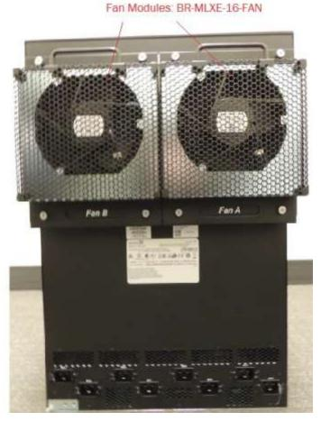
Figure 21 MLXe-16 Cryptographic Module with Chassis: BR-MLXE-16-MR2-M-AC (AC Power Supply)
