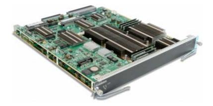
The ASA-SM, part number WS-SVC-ASA-SM1-K9, is a high performance security service module (SM) housed in the Catalyst 6500 with Sup2T chassis. It will serve as the next generation for the existing Firewall Service Module (FWSM).
