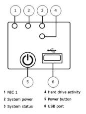
Figure 12 - \$2008, \$3008, and \$4016 Control Panel
