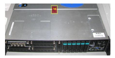
Figure 18 - Tamper-Evident Seal Application Position (\$5032 / \$6032 - Top)
