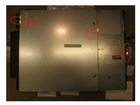
Figure 16 - Tamper-Evident Seal Application Positions (\$4016)
