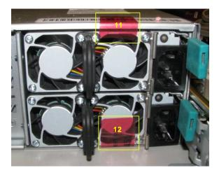
Figure 19 - Tamper-Evident Seal Application Positions (\$5032 / \$6032 - Rear)
