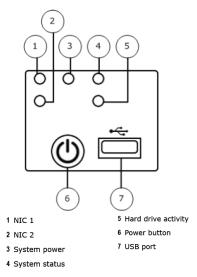
Figure 13 - S5032 and S6032 Control Panel
