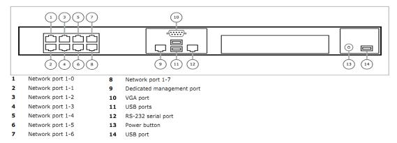
Figure 8 - Front Panel Features and Indicators for \$2008
