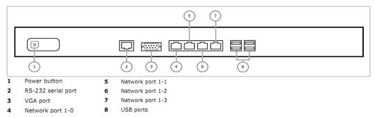
Figure 7 - Front Panel Features and Indicators for \$1104
