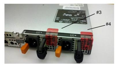
Figure 21 - I 100F Tamper-Evident Seal Application Positions (Power Supplies)
