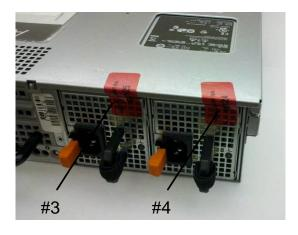
Figure 24 – 2150F Tamper-Evident Seal Application Positions (Power Supplies)
