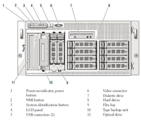
Figure 10 - 4150E Front Panel Features and Indicators
