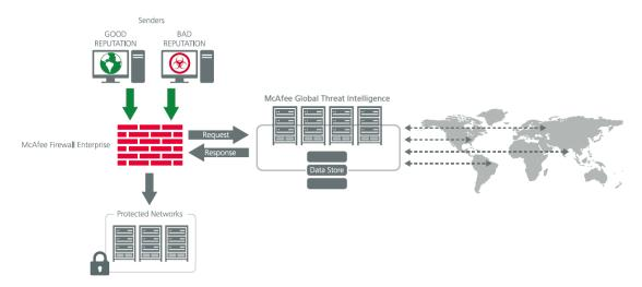
Figure I - Typical Deployment Scenario
