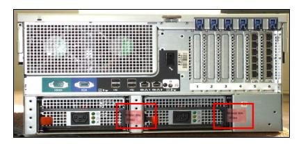
Figure 18 - 4150E Tamper-Evident Seal Application Positions (Seals #3 and #4)
