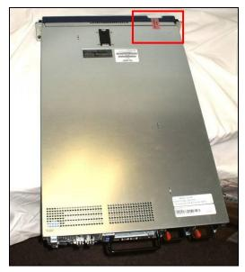
Figure 14 - 2150E Tamper-Evident Seal Application Position (Seal #1)
