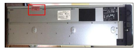
Figure 17 - 4150E Tamper-Evident Seal Application Position (Seal #2)
