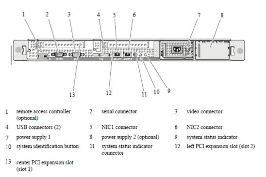
Figure 6 - I 100E Back Panel Features and Indicators
