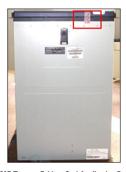
Figure 16 – 4150E Tamper-Evident Seal Application Position (Seal #1)
