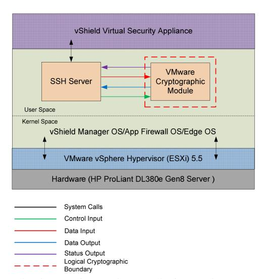
Figure 3 - VMware Cryptographic Module Logical Cryptographic Boundary
