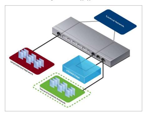
Figure I - vShield Edge Deployment Diagram
