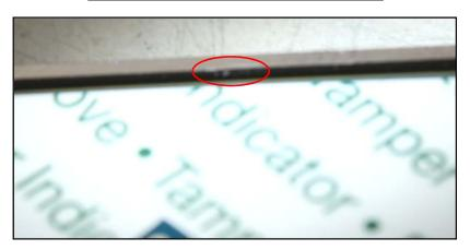
• PCB looks deformed and does not sit evenly. Red border (bottom) illustrates a tampered drive as compared to the un-tampered drive in the green border (top).
