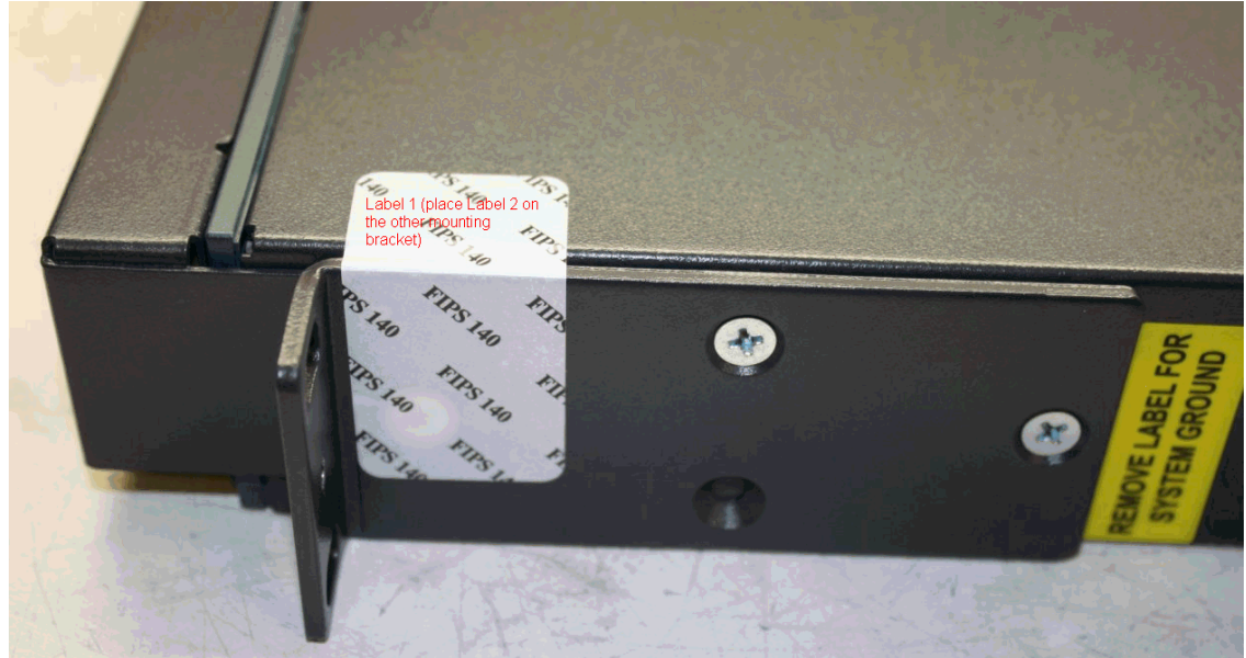
Figure 2 Placement of Tamper-evident Labels on Mounting Brackets
