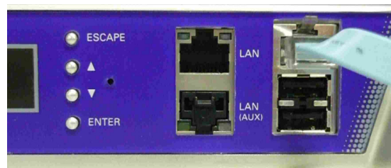
Figure 12 – Blocked LAN (AUX) RJ45 close-up
