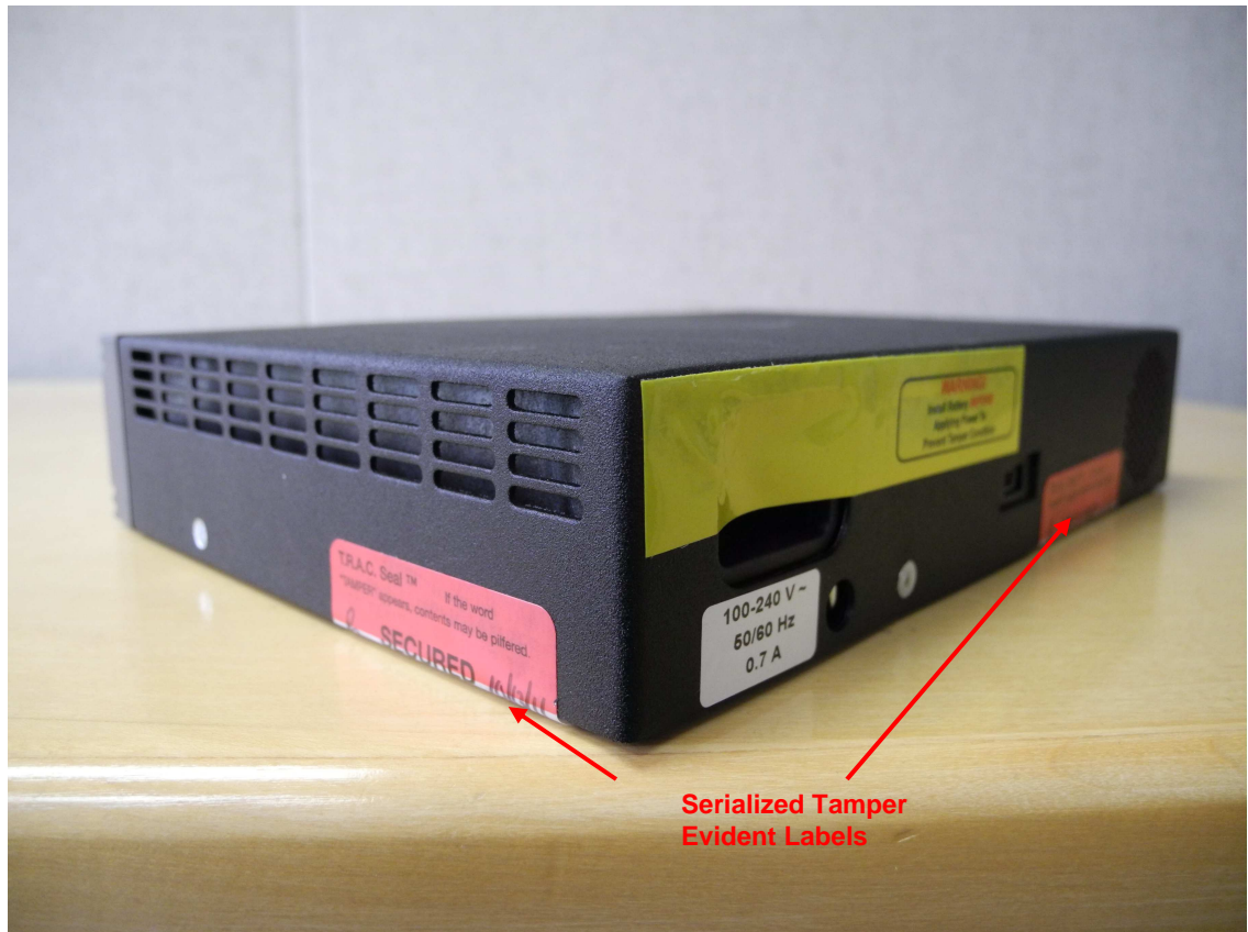
Figure 3-1. Use of Serialized Tamper Evident Labels on Luna G5
