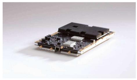
Figure 7 – iConnex e850MP-FIPSL2 Satellite Router Board (Top)
