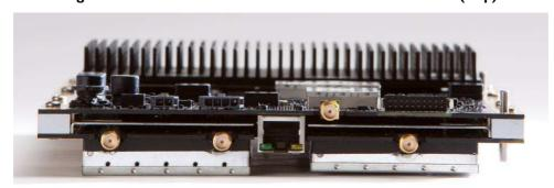
Figure 8 - iConnex e850MP-FIPSL2 Satellite Router Board (Top)
