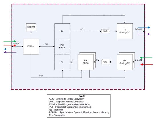
Figure 2 - Cryptographic Module Block Diagram
