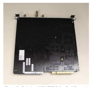
Figure 10 - Evolution eMID1-FIPSL2 Line Card (Bottom)
