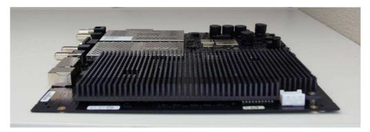
Figure 5 – iConnex e800-FIPSL2 Satellite Router Board (Top)
