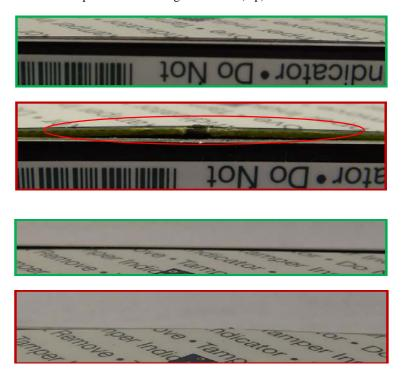
Upon discovery of tamper evidence, the module should be removed from service.
