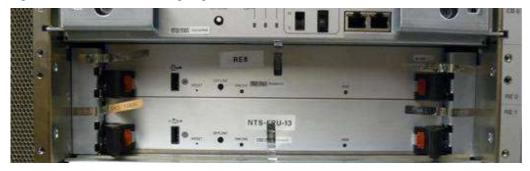
Figure 9A. T1600 FIPS Physical Boundary- T1600 Chassis RE-A-2000 in slots marked as RE1 and RE0, and Control Board in slot marked as CB0
