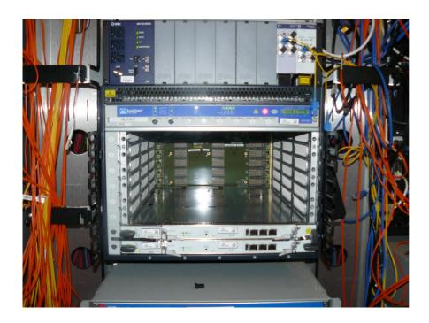
Figure 8. MX960 with Routing Engine
