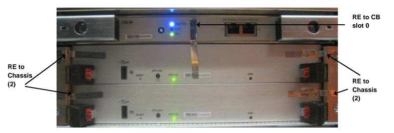
The M320 houses the RE-A-2000-4096. The physical boundary is the M320 chassis containing two routing engine units mounted next to a control board and sealed in place with five (5) tamper evident labels. The label placement for the physical boundary is identified in the figure above. Note that the additional slots of the M320 chassis are not part of the physical boundary, and the boundary traces the two routing engine units mounted next to a control board and the inside of the M320 chassis.
