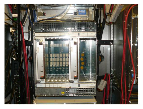
Figure 5. M320 with Routing Engine
