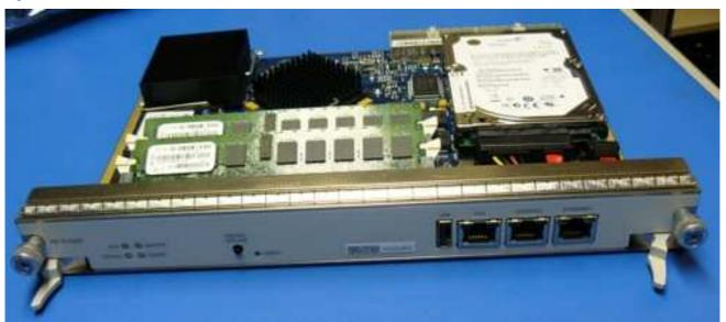
Figure 4. M120 with Routing Engine
