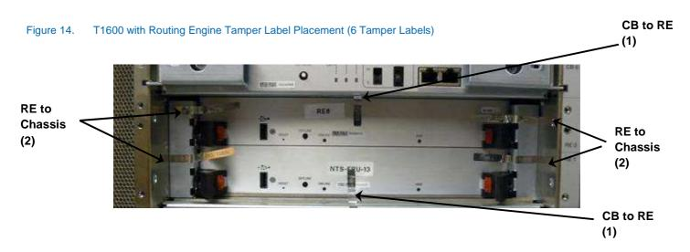
Alternate View - T1600 with Routing Engine Tamper Label Corner Placement for CB to RE Figure 15.
