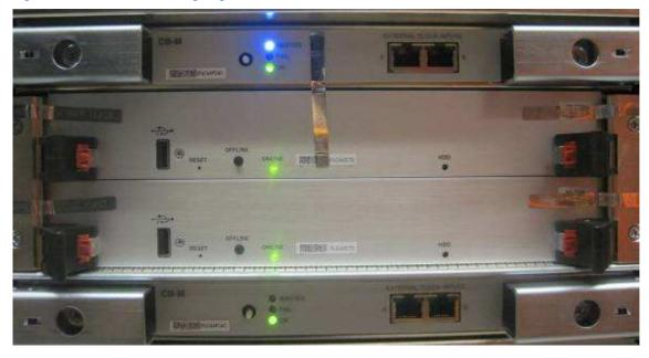
Figure 5A. M320 FIPS Physical Boundary- M320 Chassis, Routing Engine RE-A-2000 in slots marked as RE0 and RE1 and Control Board in slot marked as CB0
