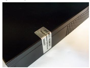
At the factory the serialized tamper evident seal shall be applied as follows::
