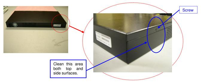
3. Identify the location to attach the label. Take note of the location of the screw head and the small hole. The label spans across rear and top panels, completely covering screw head. Note: Ventilation holes are not covered by label as shown. The minimum temperature for application is +50F.
