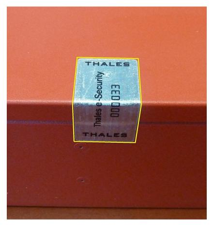
Figure 5 – Tamper Evident Label Close-Up (outlined in yellow for emphasis)
