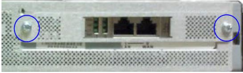
Figure 13 NIC Card Faceplate Installation
