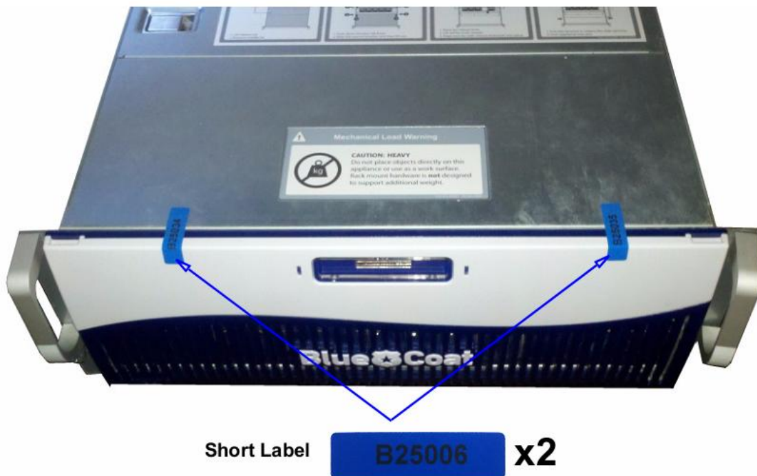
Figure 15 Front Bezel Label Application Points
