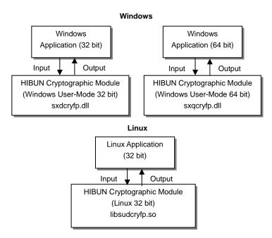
Figure 2: Relations between the HIBUN Cryptographic Module and OS
