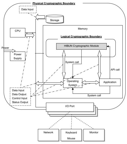
The cryptographic library module does not input data from Operating System or output data to Operating System.
