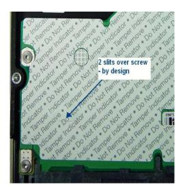
Security label over screws at indicated locations is missing or penetrated,
