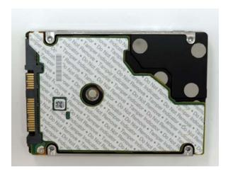
• Security labels on side of drive to provide tamper-evidence of HDA cover removal,
