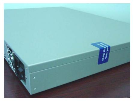
Figure 15: FortiGate-800 external enclosure seal
