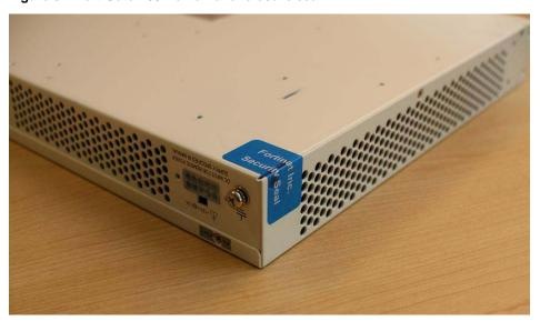
Figure 9: FortiGate-300A and 300A-HD external enclosure seal
