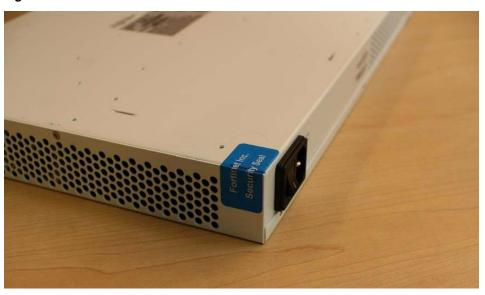
Figure 7: FortiGate-200B external enclosure seal
