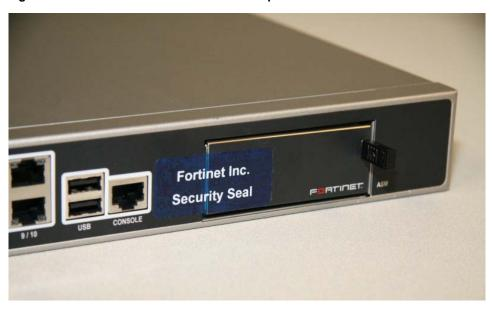
Figure 11: FortiGate-310B and 311B AMC faceplate seal
