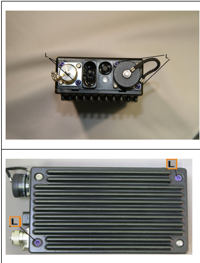
Fig 8.1 ME3-24 module views with 'loctite' compound over screws and switch mounting (blue color / L label) for tamper evidence and resistance. (views not to scale )
