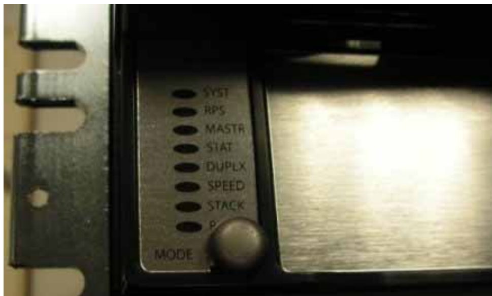
Figure 2 Placement of cap on the mode button
