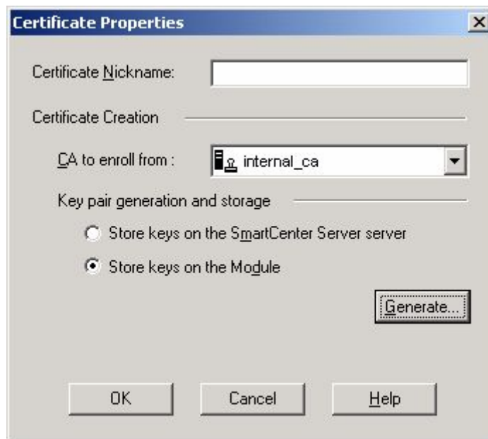
Figure 9 – Configuring the module to generate RSA keys with DKM on a per-certificate basis
